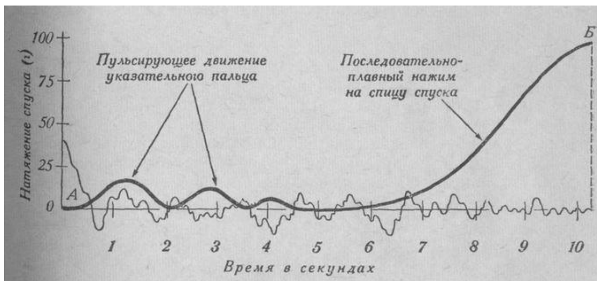
Fig. 242 - Schematic diagram of the most appropriate trigger control with an accelerator when shooting from a rifle while standing and kneeling and from a free pistol
