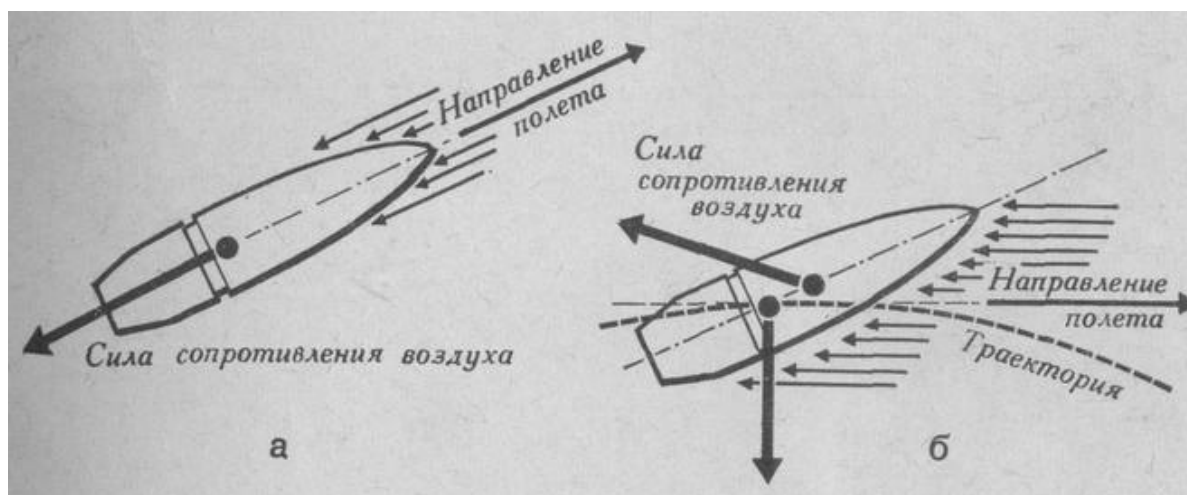
Fig. 43 - The effect of air resistance on a bullet:
