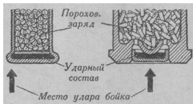
Fig. 26 - Impact composition (initiating explosives) in rifle cartridges
